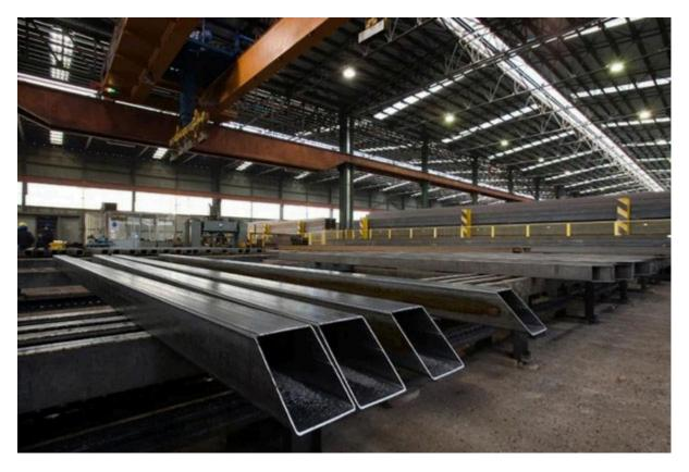
Steel columns sit on the assembly line at a Manni Sipre warehouse.
